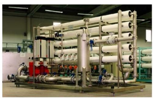
The Lofsdalen nanofiltration plant consists of 10 pressure vessels, each containing four FILMTEC™ elements. The vertical metal cylinder is the housing for the cartridge filters. The two vertical boxes at the left are the frequency controllers for the recirculation pumps below. All pipework is stainless steel. (Photo courtesy of HOH Water Technology.)
